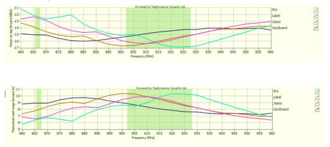
Sensitivity&Read Rang Test power: 4W EIRP
