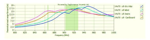
Sensitivity&Read Rang Test power: 4W EIRP
