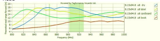
Sensitivity&Read Rang Test power: 4W EIRP
